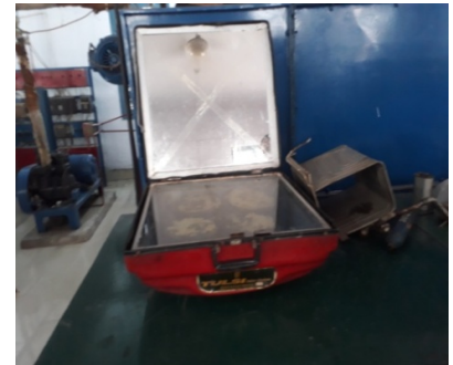
Solar Energy Lab (Thermal Performance of Solar Cooker)
