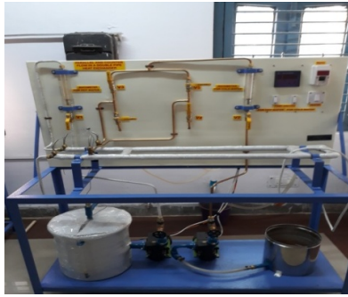
Heat Transfer Lab (Double Pipe Heat Exchanger setup)
