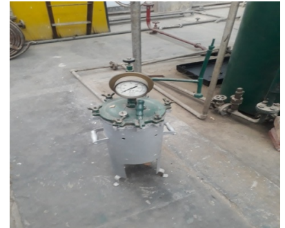
Steam Power Lab (Mercets Boiler for Thermocouple Calibration)
